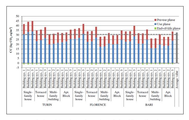
Fig. 3 - Annual values of the indicator Climate Change (CC) in different life cycle stages, for different categories of buildings, located in three Italian cities and equipped with three building system solutions (1 = only heating with underfloor panels, 2 = only heating with radiators, 3 = heating with underfloor panels & cooling with multi-split systems).
