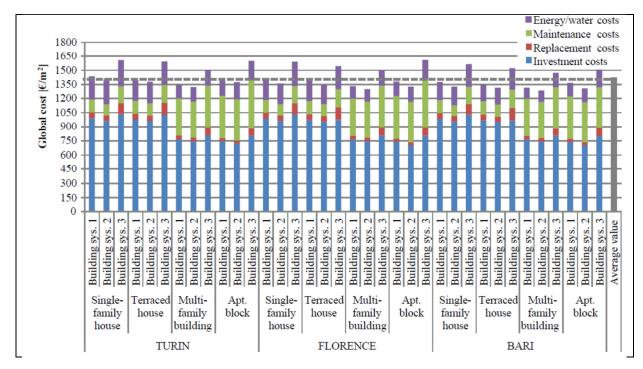
Fig.4 - Values of the global cost for different categories of buildings, located in three Italian cities and equipped with three building system solutions (1 = only heating with underfloor panels, 2 = only heating with radiators, 3 = heating with underfloor panels & cooling with multi-split systems).
