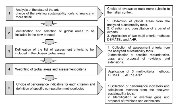
Fig. 1 - Methodological steps for the definition of the structure of the new protocol.
