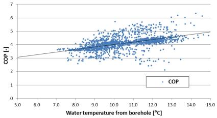
*Fig. 4 - Hourly average COP related to hourly average water temperature from boreholes. <u>Heating</u> <u>mode</u>*
