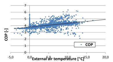
Fig. 5 - Hourly average COP related to hourly average external air temperature. Heating mode
