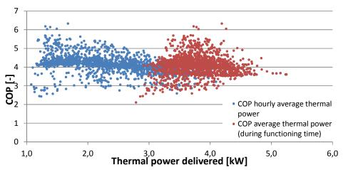
*Fig. 6 - Average COP related to themal power delivered to the plant: hourly average value in blu and average value, calculated only when the heat pump is functioning, in red. <u>Heating mode</u>*
