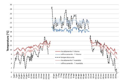
Fig. 3 - Daily average temperature of external air and of water from boreholes
