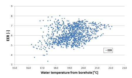
Figure 7: Hourly average EER related to hourly average water temperature from boreholes. <u>Cool-ing mode</u>
