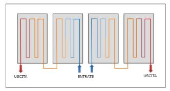
Fig. 9 – Hydraulic connection of the PV-T panels
