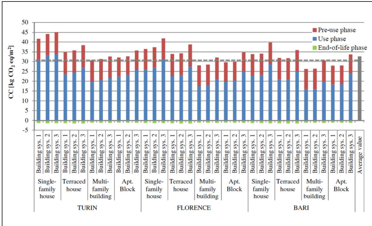
Fig. 3 - Annual values of the indicator Climate Change (CC) in different life cycle stages, for different categories of buildings, located in three Italian cities and equipped with three building system solutions (1 = only heating with underfloor panels, 2 = only heating with radiators, 3 = heating with underfloor panels & cooling with multi-split systems).
