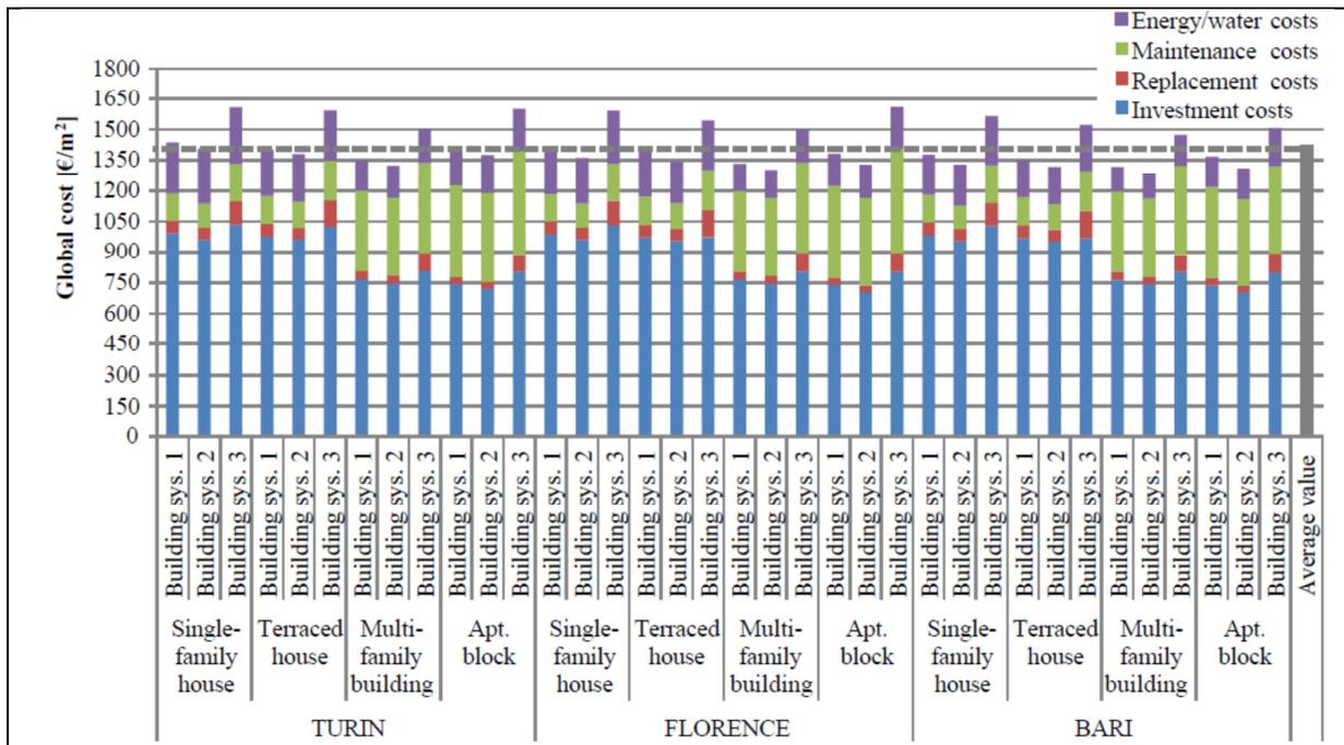
Fig.4 - Values of the global cost for different categories of buildings, located in three Italian cities and equipped with three building system solutions (1 = only heating with underfloor panels, 2 = only heating with radiators, 3 = heating with underfloor panels & cooling with multi-split systems).
