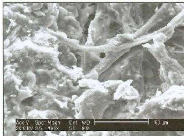
Electron microscope image showing fibers, dust, and other deposited material on a residential air conditioner coil.
