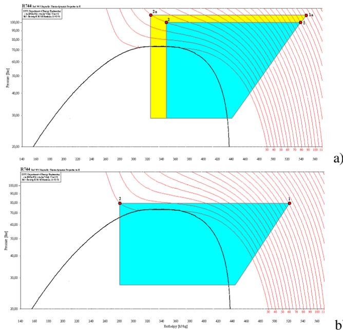
Figure 2 – Thermodynamic cycles for two different water temperatures at gas cooler inlet. The inlet water temperature is equal to 40 °C in case a) and 25 °C in case b). From (Vio, 2013).
