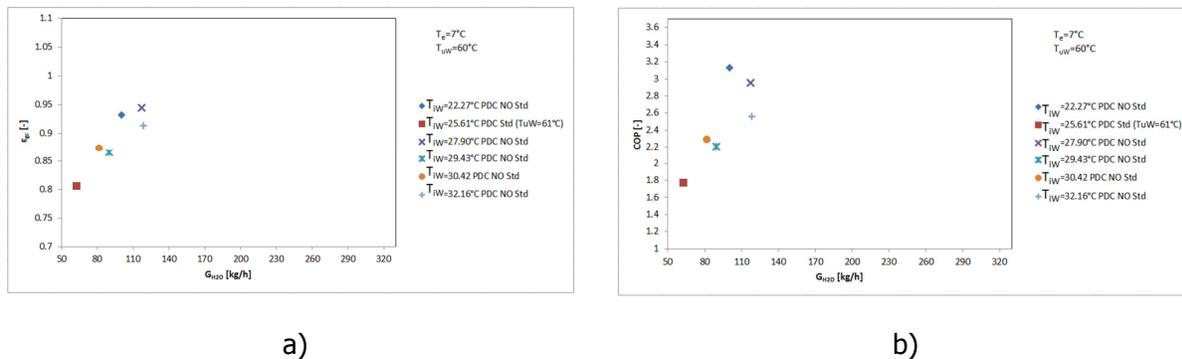
Figure 11 - For  $T_e = 7\text{ °C}$  and  $T_{uw} = 60\text{ °C}$  a) Efficiency of the gas cooler,  $\varepsilon_{gc}$ , b) COP of the heat pump as a function-of water flow.
