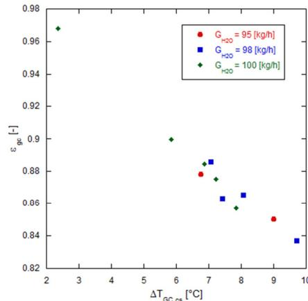
Figure 12 - Efficiency of the gas cooler,  $\varepsilon_{gc}$ , as a function of the temperature difference between the temperature of CO<sub>2</sub> at gas cooler outlet and the water temperature at gas cooler inlet.
