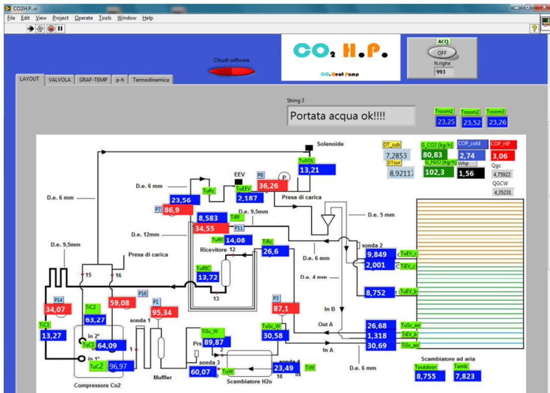
Figure 7 - Instrumented heat pump system layout. From (Boccardi, 2012).
