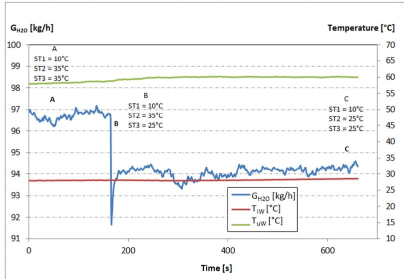
Figure 16 - Trends of parameters measured on the water side of the heat exchanger during the time for  $T_e = -11$  °C and  $T_a = 19$  °C and with electronic modulating valves.
