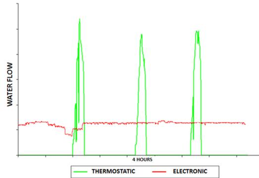
Figure 4 – Comparison of water flow distribution in terminal heating unit with high water content in the case of traditional thermostatic valve and in the case of electronic valve.
