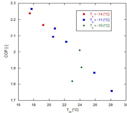
Figure 10 - Heat pump COP trend as a function of the water temperature at gas cooler inlet,  $T_{iw}$ , for three values of outside air temperature,  $T_e$ .
