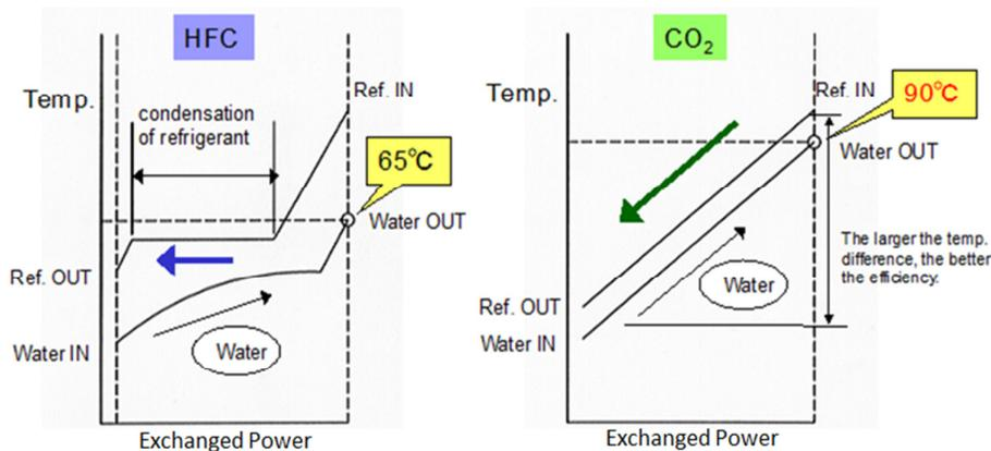
Figure 1 – Difference between the temperature profiles in a HFC condenser and in a CO<sub>2</sub> gas cooler in a heat pump for heating water.
