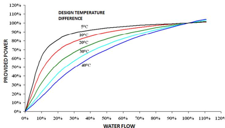
Figure 3 – Variation of output power from a heating terminal unit to vary the temperature difference between inlet and outlet at nominal design conditions, valid for a value of the inlet water temperature equal to 75 °C.
