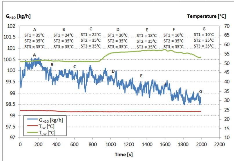
Figure 14 – Trends of parameters measured on the water side of the heat exchanger during the time and with electronic modulating valves for  $T_e = -10\text{ °C}$  and  $T_a = 18\text{ °C}$ .
