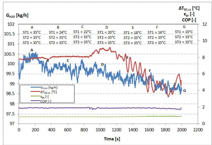
Figure 15 - Heat pump performances trend during the time and with electronic modulating valves for  $T_e = -10\text{ °C}$  and  $T_a = 18\text{ °C}$ .
