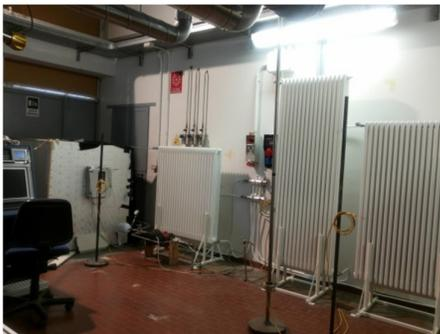
Figure 5 - Test facility with CO<sub>2</sub> heat pump with heating terminal units of high temperature difference.
