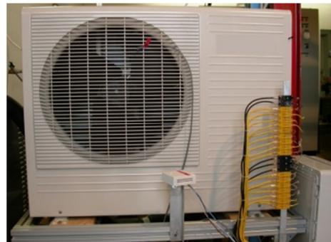
Figure 6 – CO<sub>2</sub> heat pump.
