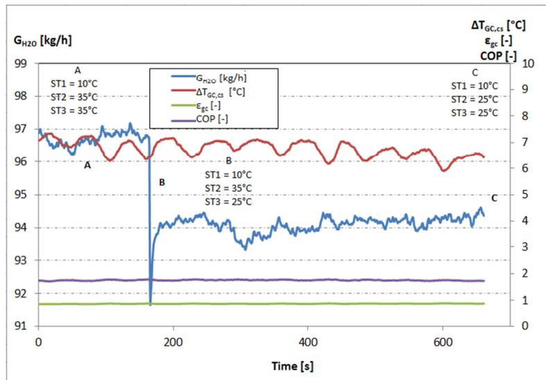
Figure 17 – Heat pump performances trend during the time and with electronic modulating valves for  $T_e = -11$  °C e  $T_a = 19$  °C and with electronic modulating valves.
