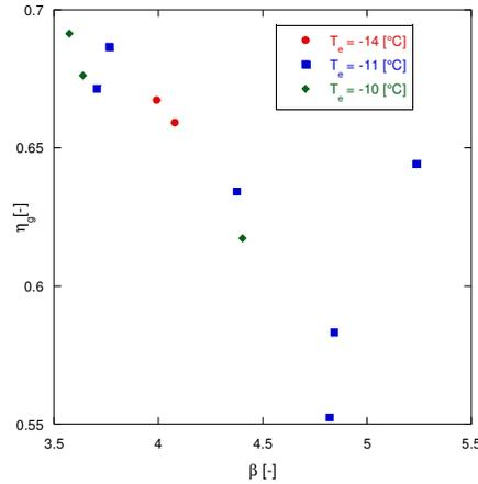
Figure 9 - Compressor overall performance  $\eta_g$  trend as a function of the compression ratio,  $\beta$ , for three values of outside air temperature,  $T_e$ .
