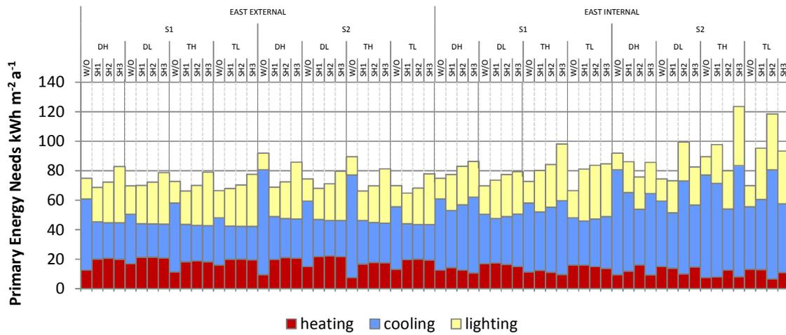
Figure 12 – Primary energy needs in the different configurations for East orientation.
