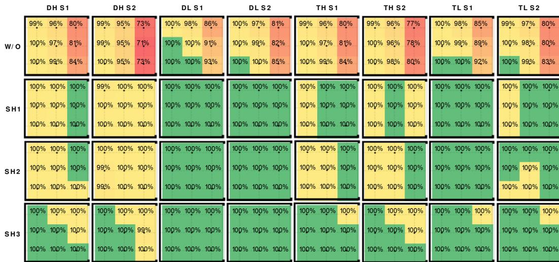
Figure 6 – Visual Comfort Availability distribution for East orientation and external shades. Each square represents the plant of the office with the window on the East side (symbols are explained in Table 1).
