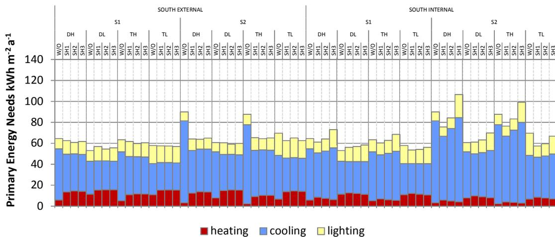
Figure 13 – Primary energy needs in the different configurations for South orientation.
