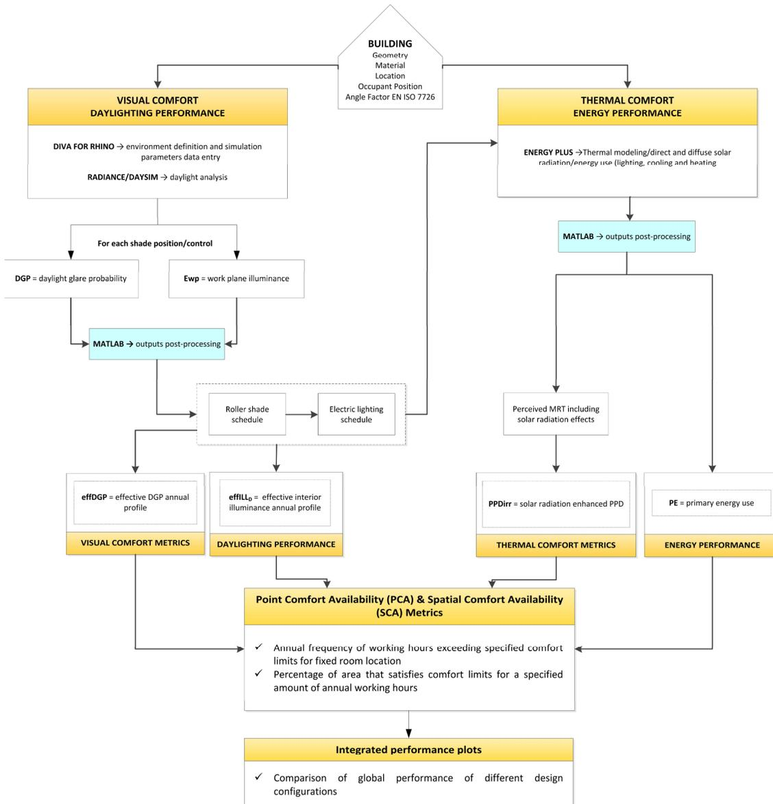
Figure 1 – Calculation procedure of the global performance of the considered building modules.
