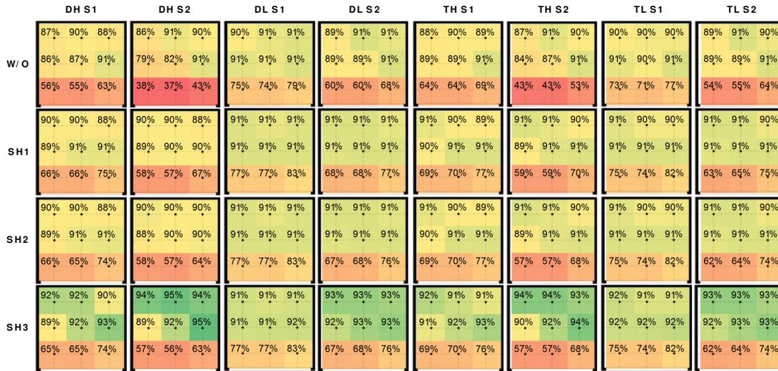
Figure 7 – Visual Comfort Availability distribution for South orientation and external shades. Each square represents the plant of the office with the window on the South side (symbols are explained in Table 1).
