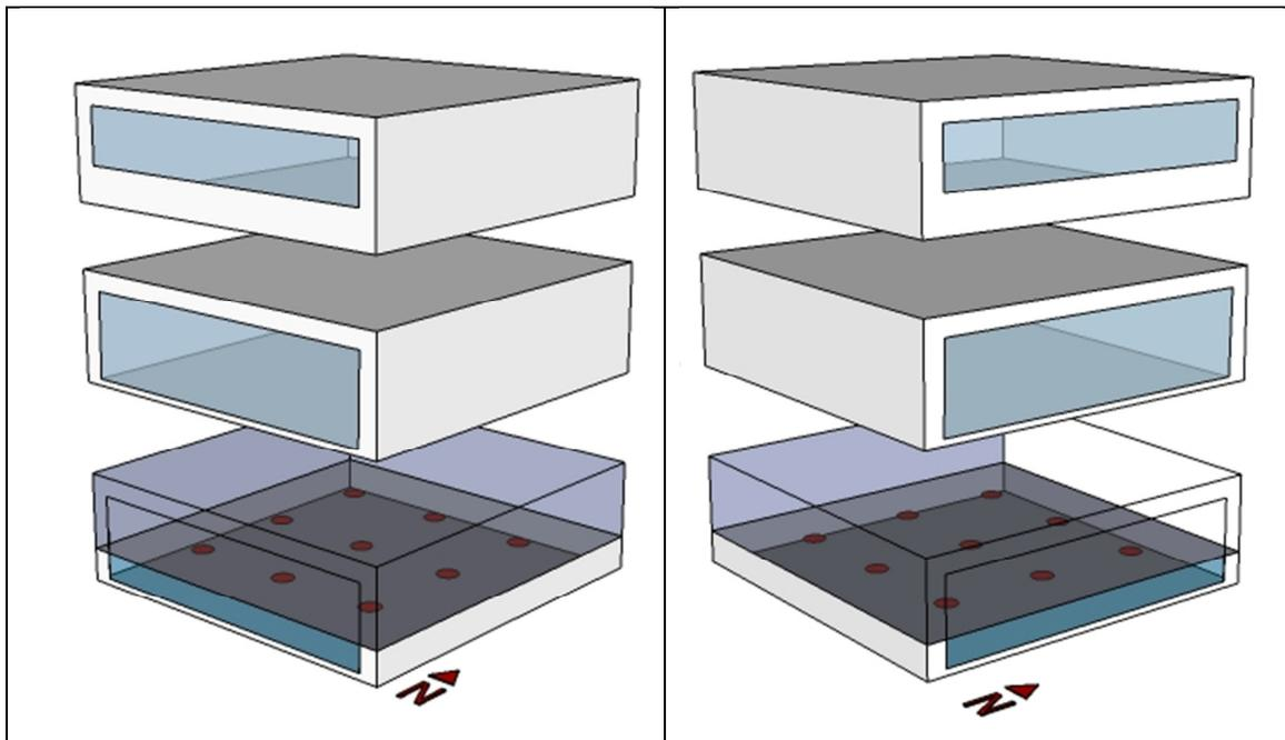
Figure 2 – Sketch of the simulated office building: configuration with S1 windows' size (small) – above; with S2 windows' size (large) – middle; section plane with the position of the grid of points considered in the comfort analysis – below.
