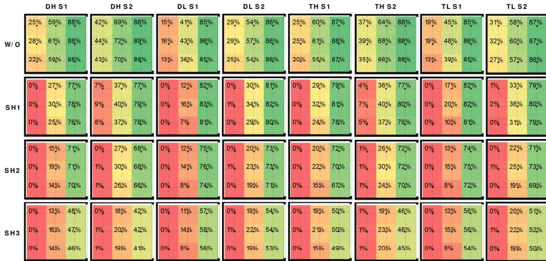
Figure 3 - Daylight Autonomy distribution for East orientation and external shades. Each square represents the plant of the office with the window on the East side (symbols are explained in Table 1).
