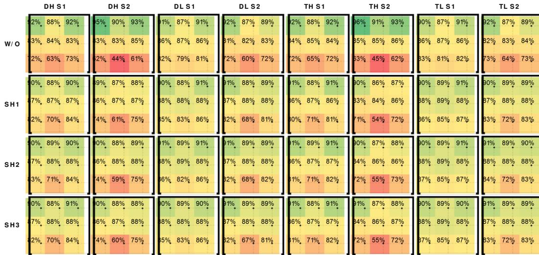
Figure 9 – Thermal Comfort Availability distribution for South orientation and external shades. Each square represents the plant of the office with the window on the South side (symbols are explained in Table 1).
