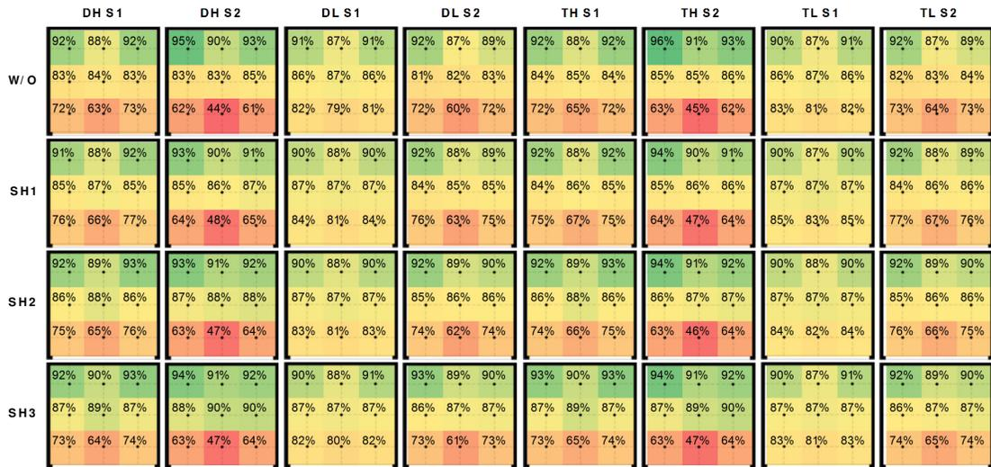
Figure 10 – Thermal Comfort Availability distribution for South orientation and internal shades. Each square represents the plant of the office with the window on the South side (symbols are explained in Table 1).
