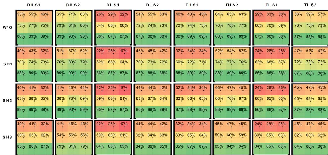
Figure 4 - Daylight Autonomy distribution for South orientation and external shades. Each square represents the plant of the office with the window on the South side (symbols are explained in Table 1).
