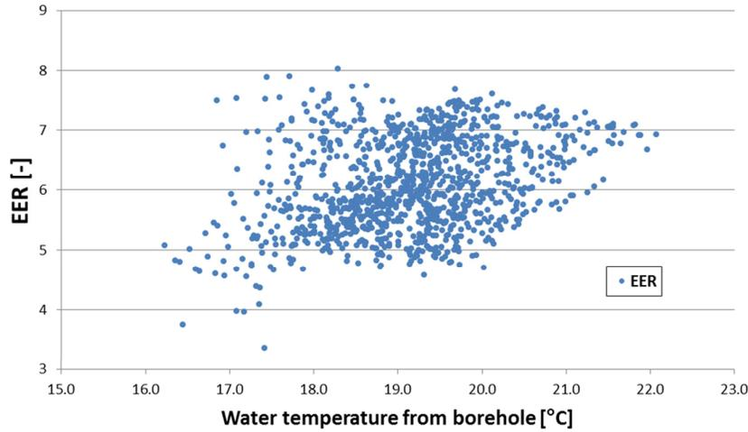
Figure 7: Hourly average EER related to hourly average water temperature from boreholes. Cooling mode
