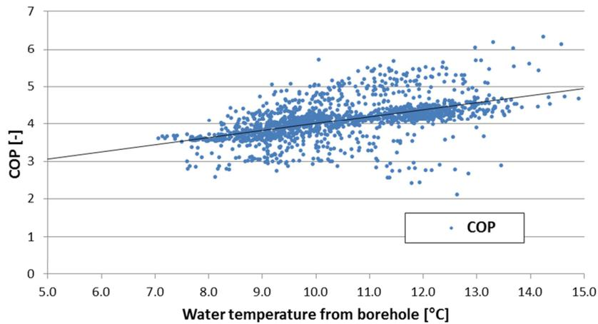
Fig. 4 - Hourly average COP related to hourly average water temperature from boreholes. Heating mode
