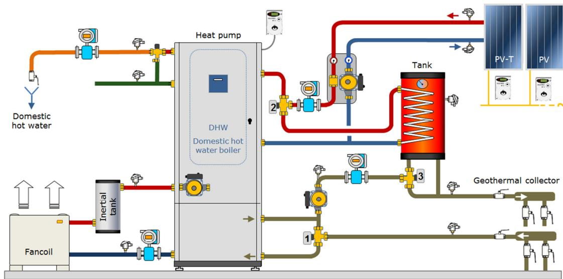
Fig. 1 - Plant scheme and monitoring system
