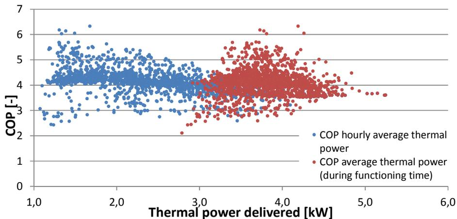
Fig. 6 - Average COP related to thermal power delivered to the plant: hourly average value in blu and average value, calculated only when the heat pump is functioning, in red. Heating mode
