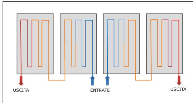
Fig. 9 – Hydraulic connection of the PV-T panels
