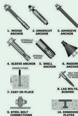
Figure 130: Types of anchors.
