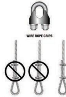
Figure 154: Wire rope grip assemblies.
